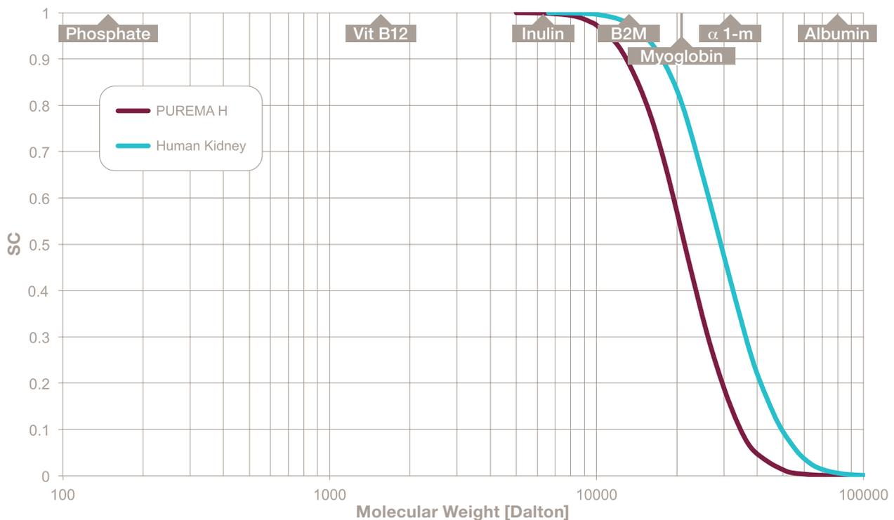
Sieving coefficients are tested per DIN 58353: 5% bovine albumin-containing saline; flow conditions are  $Q(B)=200\text{mL}/\text{min}\cdot\text{m}^2$  and  $Q(F)=30\text{mL}/\text{min}\cdot\text{m}^2$  for high flux membranes.
